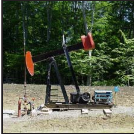
An active pump, which aids in filling the gas/oil tanks.
